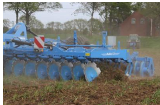
Figur 6.13: Lemken Rubin 12 - aggressive 736 mm tallerkner. Foto: Lemken
